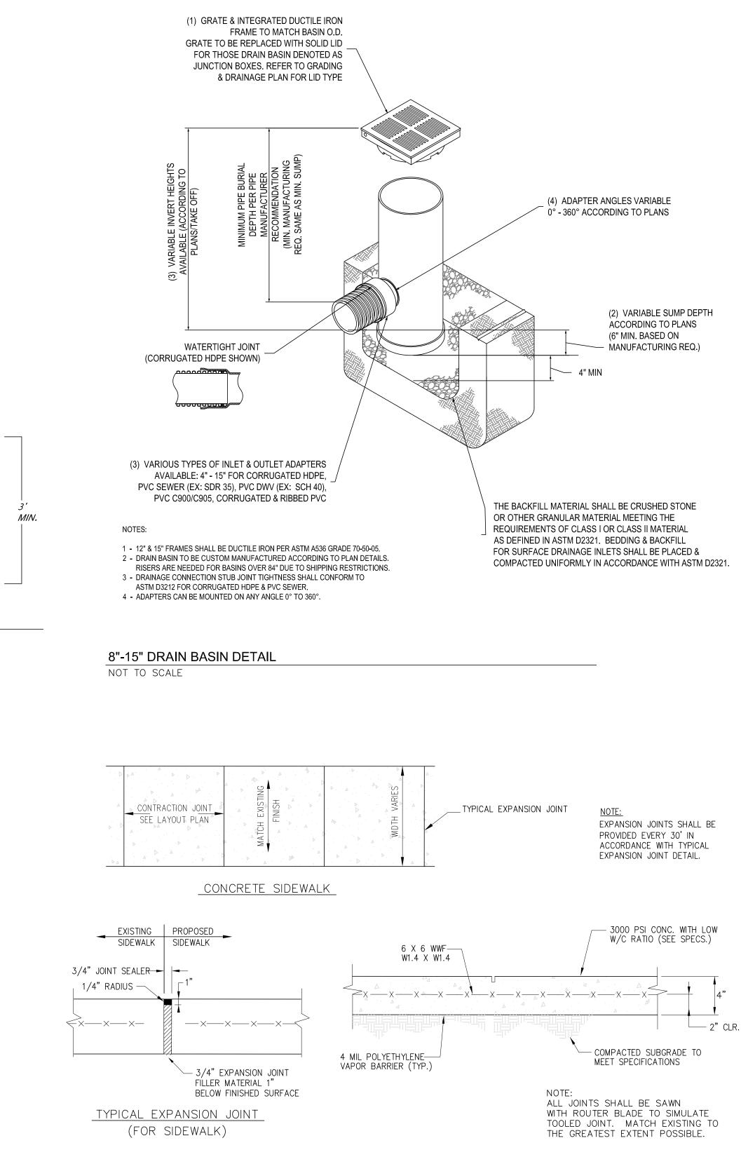
1. CONCRETE SCORING 5' O.C. AND EXPANSION JOINTS AT 30' O.C. OR MATCH EXISTING SIDEWALK JOINT SPACING.
